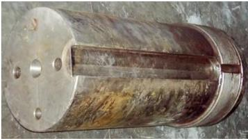
Premature failure of integral pinion shaft was reported at a cement mill. The shaft failed after service life of approximately 15,000 hours (625 days) against intended design life of 30 years. The shaft is made from EN 10083-1 (1991) 30CrNiMo8 with through hardened and tempered to achieve 310-335 BHN. The shaft rotates at 133 to 134 RPM. The failure of the shaft
