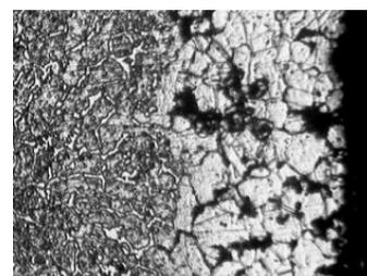
outer diameter and progressing towards ID. This magnification was done at the TCR Engineering laboratory using a Leco Image Analyser at 300X.
