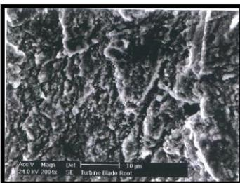
Scanning Electron Microscopy (SEM): Fracture surface kept under SEM show multiple origins of the fracture and clearly shows progressive mode of failure. Fig. suggest rubbing of the metal surface where the failure had occurred.
