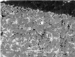
Upon SEM examination conducted by engineers at TCR, it revealed presence of inter-granular cracks and presence of numerous creep cavities at grain boundary. Presence of micro-cracks are observed more towards outer surface and near by crack region. Severity of cracks and cavity reduces when we move away from the main crack.
