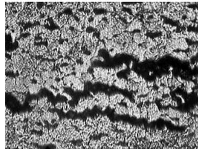
In present case the failure of tube seems to have occurred due to long term over- heating, above allowable design temperature, could be due to higher velocity of flue gas at this region or impingement of flue gases on tube surface facing flue gas or improper steam flow.
